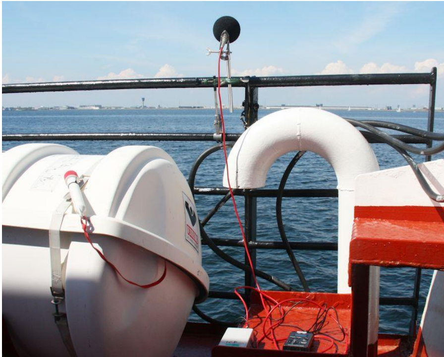
Figure 5 Microphone for recording of aircraft noise (Klaus Betke).
