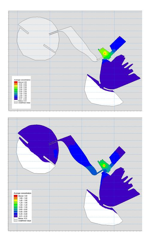
Figure 3.6 Modelled concentration of dissolved TBT in the Rødbyhavn harbour and lagoon system during model period 1. Upper figure: no connection between western harbour and Inner Lagoon (≈ present situation, baseline); lower figure: future harbour-lagoon layout with a channel connection western harbour to Inner Lagoon.
