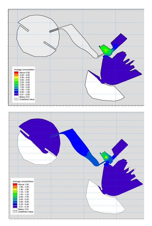
Figure 3.7 Modelled concentration of dissolved TBT in the Rødbyhavn harbour and lagoon system during model period 2. Upper figure: no connection between western harbour and Inner Lagoon (≈ present situation, baseline); lower figure: future harbour-lagoon layout with a channel connection western harbour to Inner Lagoon.
