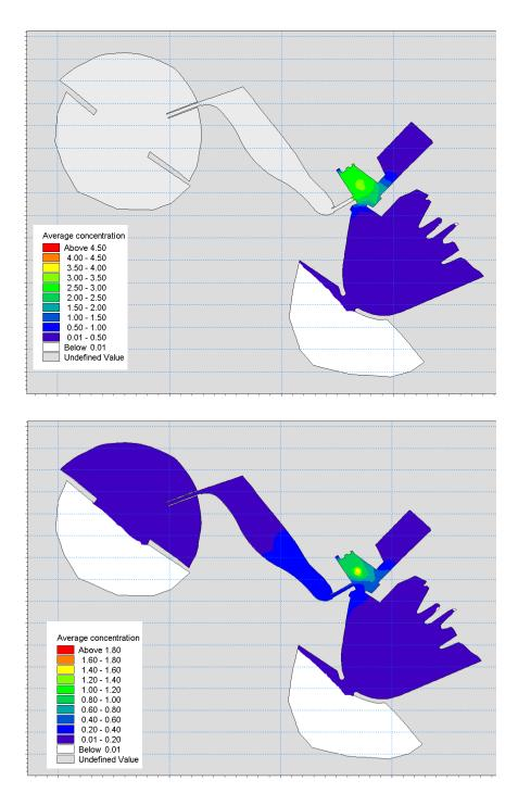
Figure 3.8 Modelled concentration of dissolved TBT in the Rødbyhavn harbour and lagoon system during model period 3. Upper figure: no connection between western harbour and Inner Lagoon (≈ present situation); lower figure: future harbour-lagoon layout with a channel connection western harbour to Inner Lagoon.
