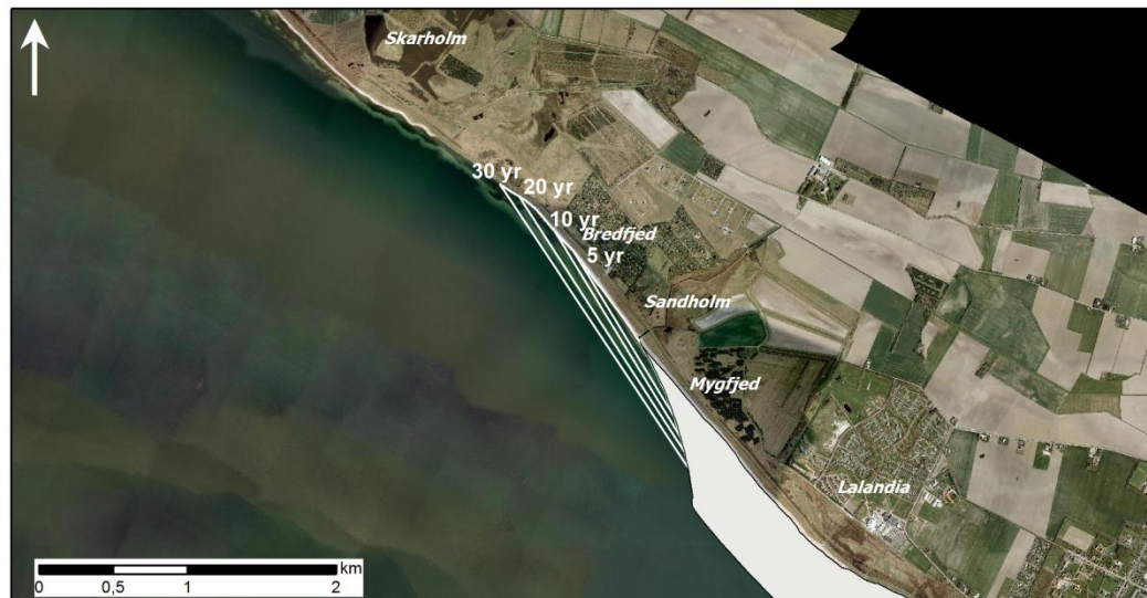
Figure 6-1 Predicted development of the shoreline west of the Lolland reclamation 0-30 years after end of construction. Aerial photo from 2009 (©COWI Orthophoto April 2009)
