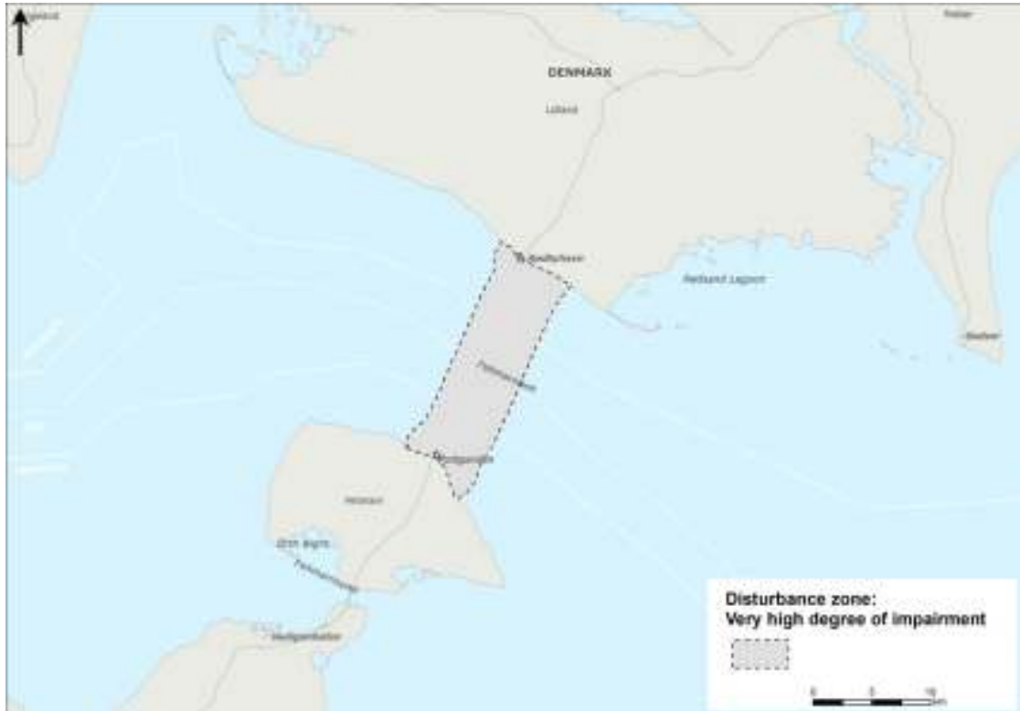
Figure 10.34 Disturbance zone of the construction activities defined as a 3 km buffer around the cable stayed bridge footprint.
