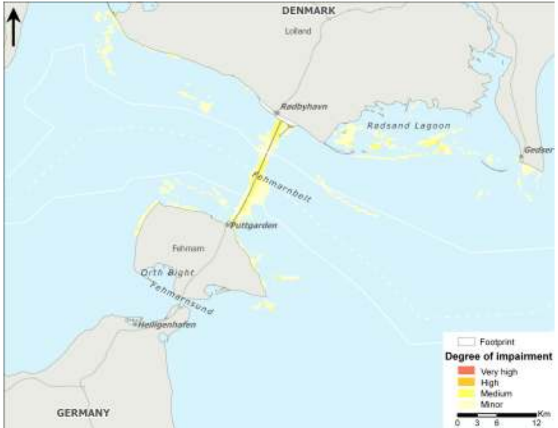
Figure 9.21 Degree of impairment for benthic fauna from sedimentation due to construction activities of an immersed tunnel (for definitions of different levels of degree of impairment see FEMA (2013d); maps taken from FEMA (2013d)).
